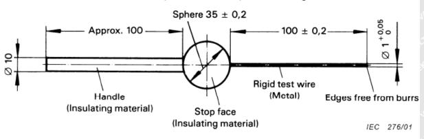
Test wire 1,0 mm diameter, 100 mm long
