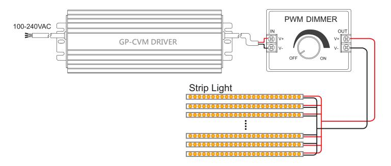
The GP-CVM series are the silent LED drivers, include connecting to the external PWM dimming controller with low noise operation.
