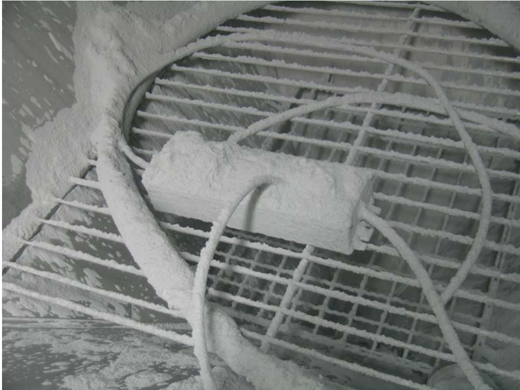
LED Driver : IPX7 Test Photo
