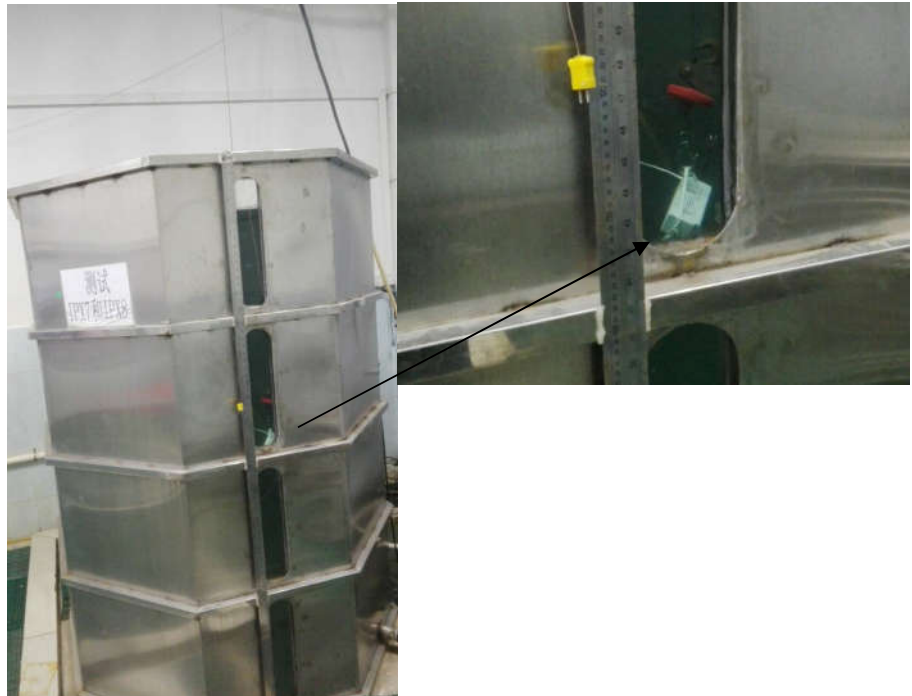
Figure .4- IPX7 testing
