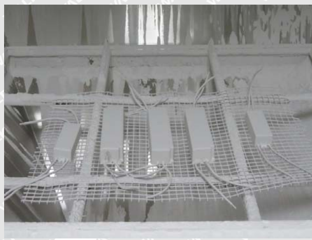
Photo 2 -- During the test of IP6X
